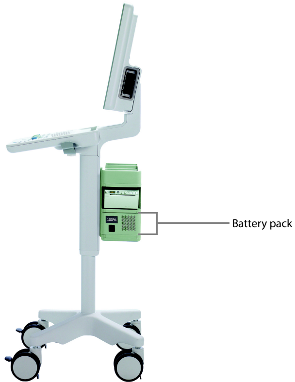
Figure 4-1. System with battery support in the backpack.
